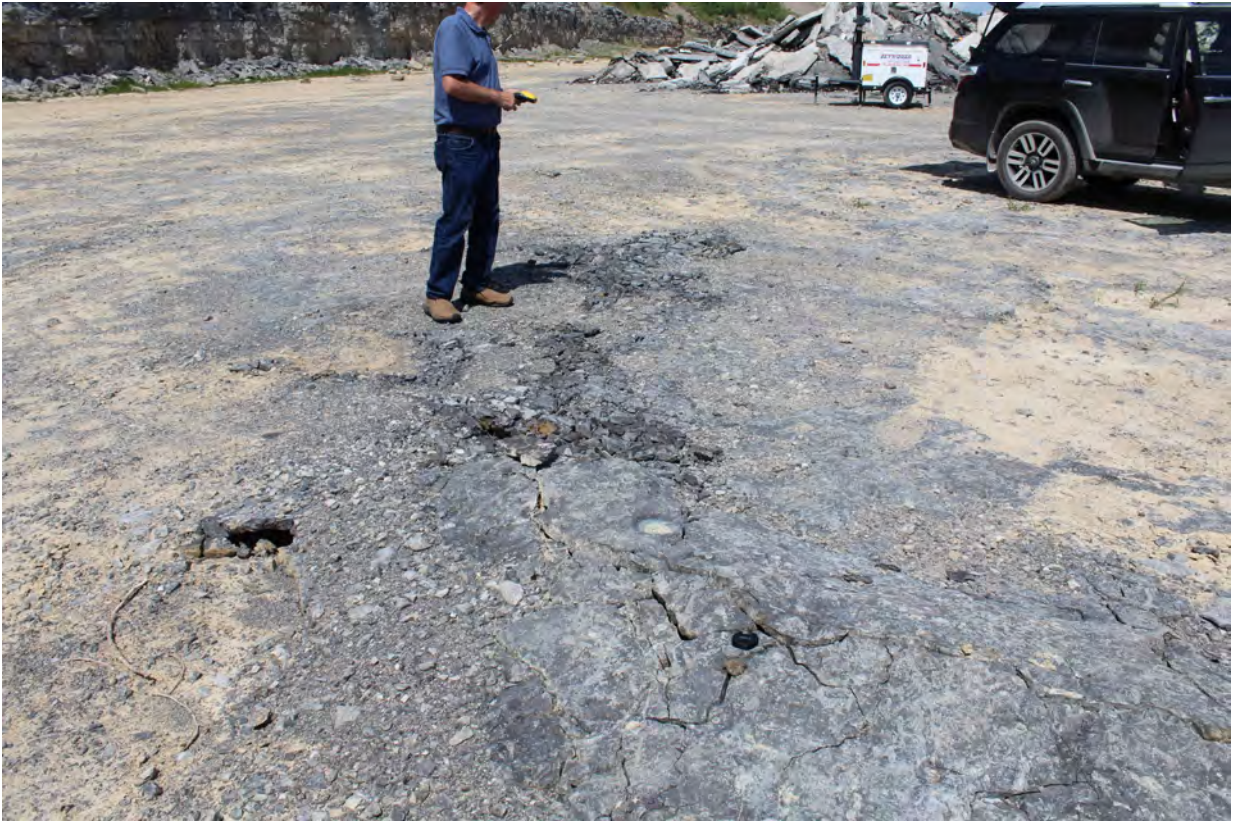
3046, 8/15/2022, by Sam Gowan: Broken rock associated with the localized rock pop-up in the County Line Stone Akron Quarry.
