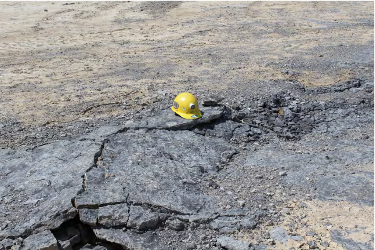
3042, 8/15/2022, by Sam Gowan: Localized rock pop-up in the County Line Stone Akron Quarry.
