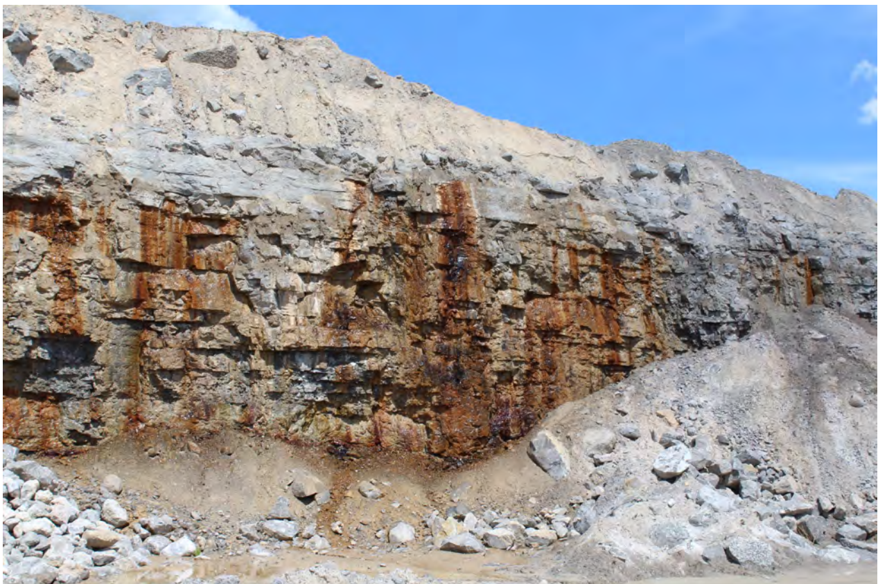
3055, 8/15/2022, by Sam Gowan: Ground water and iron staining emanating from near the base of the overburden on the north highwall of the County Line Stone Akron Quarry. The discharged ground water is pooled on the quarry floor at the base of the highwall.
