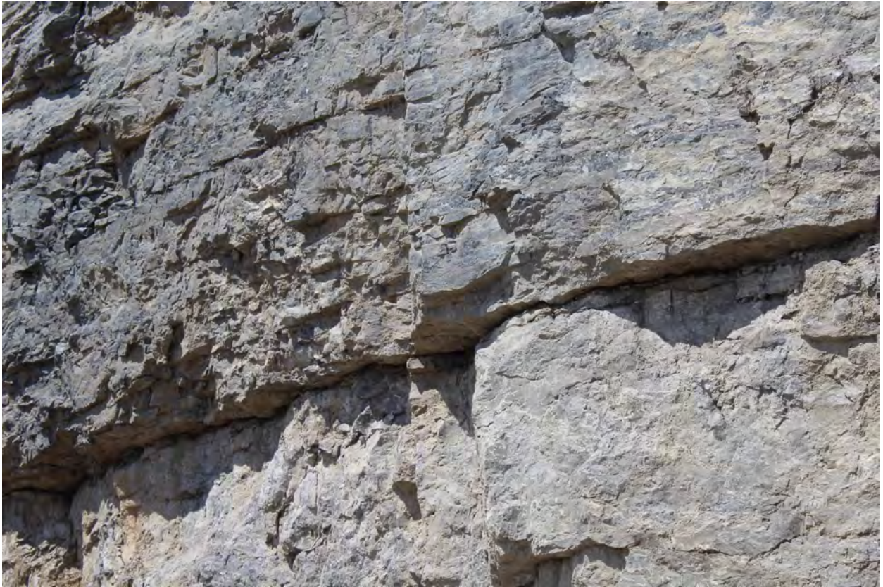
3052, 8/15/2022, by Sam Gowan: View of a secondary joint in the north rock face at the County Line Stone Akron Quarry. The joint is oriented N47°W.
