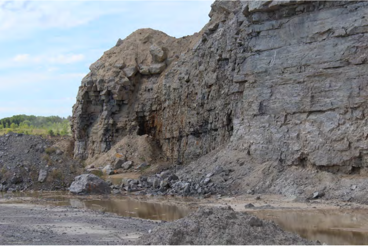
3058, 8/15/2022, by Sam Gowan: Ground water seepage and pooled ground water discharge along the north face of the County Line Stone Akron Quarry.
