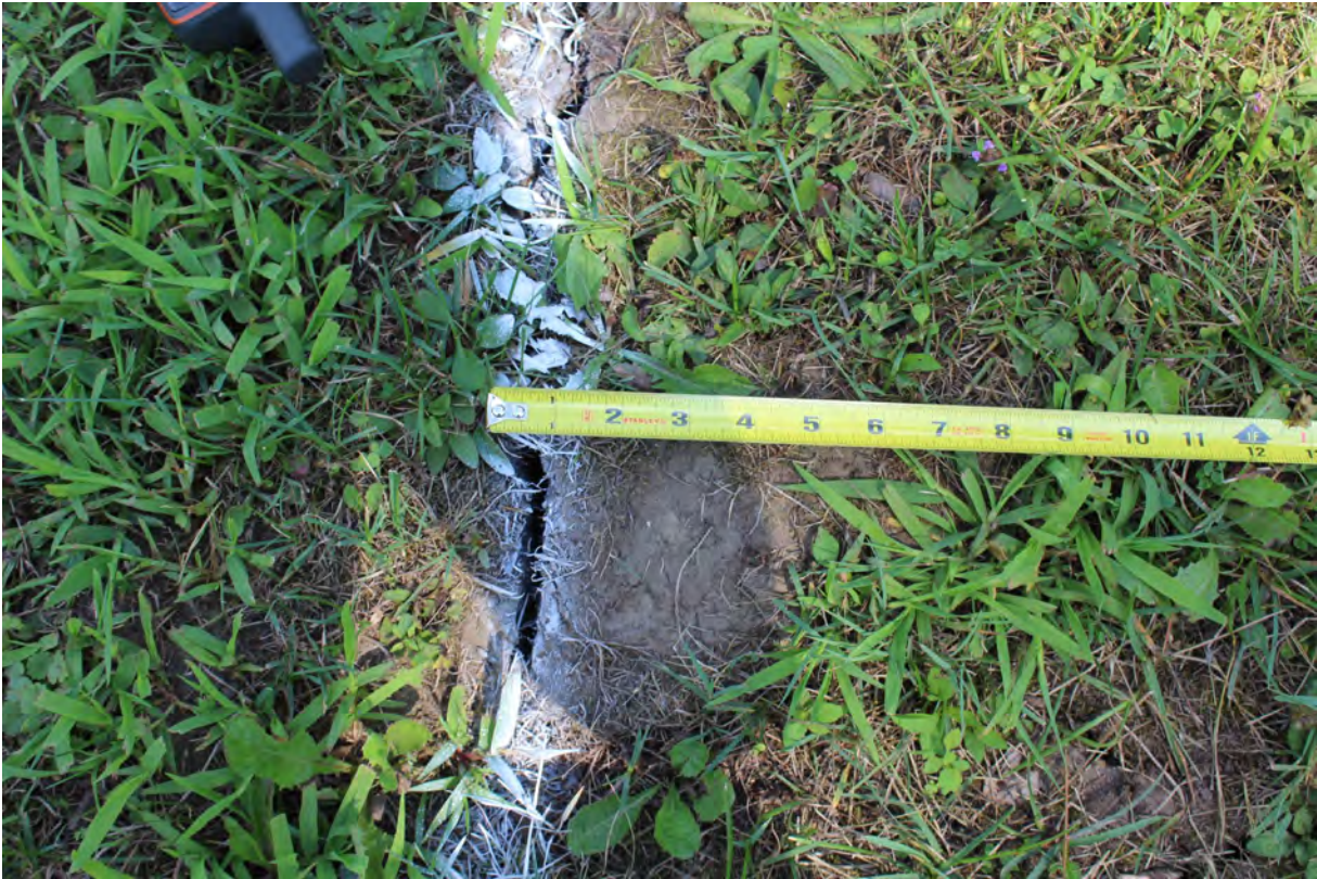
3023, 8/15/2022, by Sam Gowan: Measured aperture in fracture at Gowan location 133 (430 Scribner Road). No fractures were observed further to the south-southwest.
