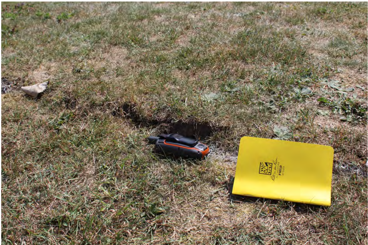
3024, 8/15/2022, by Sam Gowan: View toward the east of an apparent offset in a fracture at 440 Scribner Road (Gowan location 134). The field book is 7 inches long.
