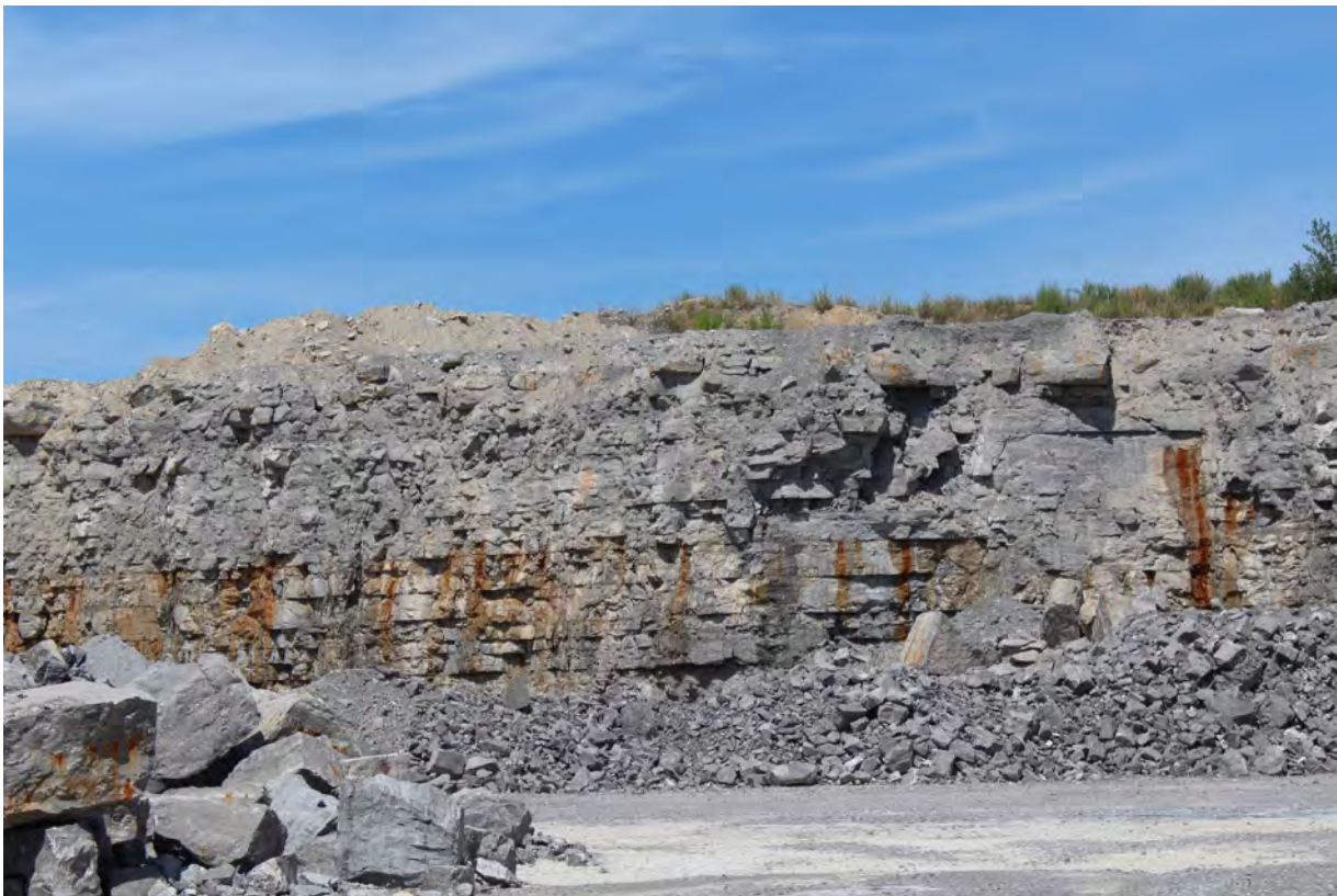
3063, 8/15/2022, by Sam Gowan: Iron staining and ground water seepage from the north highwall near the northeast corner of the County Line Stone Akron Quarry.
