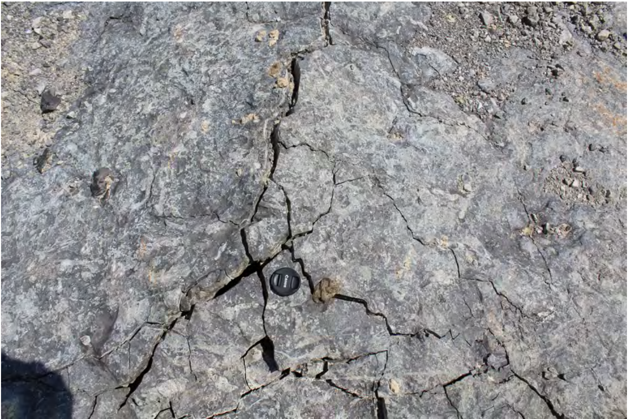
3044, 8/15/2022, by Sam Gowan: Top view of the localized rock pop-up in the County Line Stone Akron Quarry (see 3042).
