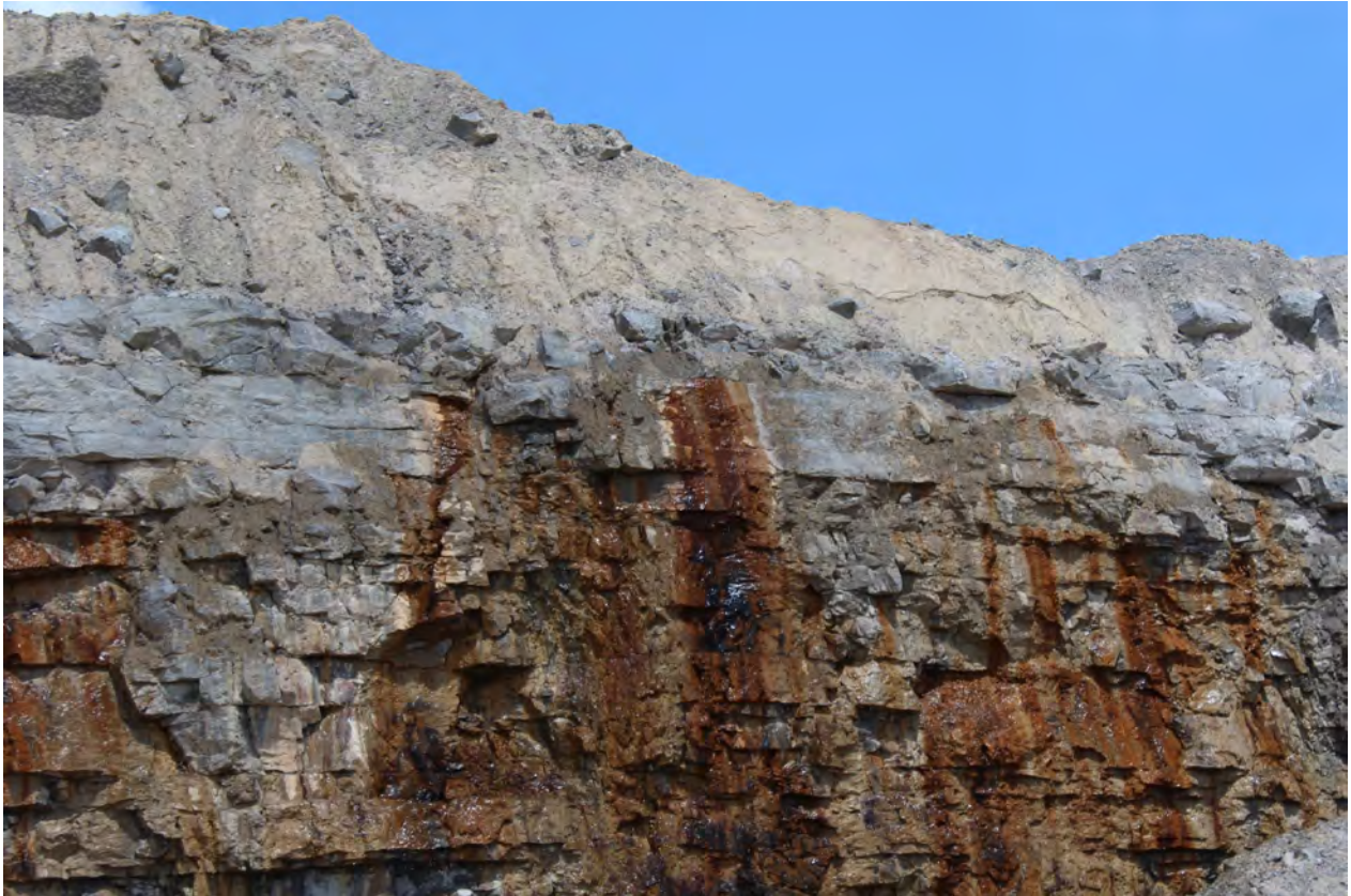
3056, 8/15/2022, by Sam Gowan: Ground water seepage from near the base of the overburden on the north face of the County Line Stone Akron Quarry.
