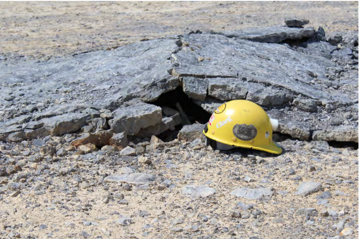
3043, 8/15/2022, by Sam Gowan: Localized rock pop-up in the County Line Stone Akron Quarry.
