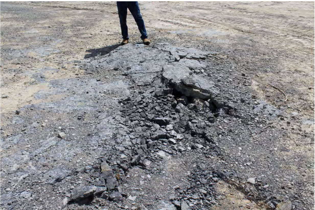
3047, 8/15/2022, by Sam Gowan: Localized rock pop-up in the County Line Stone Akron Quarry.
